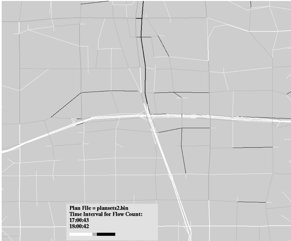
Figure 3.7: V/C-ratios in the study-area — White links mean that demand is lower than capacity ( V/C < 1 ); for gray links demand is between capacity and two times capacity ( 1 \leq V/C < 2 ); for black links demand is larger than two times capacity ( 2 \leq V/C ). The time labels (17:00-18:00) refer to an equivalent afternoon rush hour. This figure was generated using the FlashPlan visualization utility of the TRANSIMS application suite.
