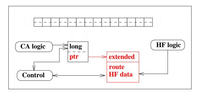
Extended data available for both models  $(CA, HF) \longrightarrow easy$  switching between models in hybrid simulation.
